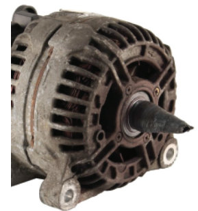
Damaged rotor shaft
